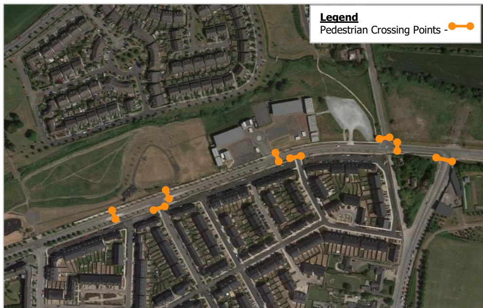
Figure 3.5: Existing Pedestrian Crossing location on Parkside Boulevard
